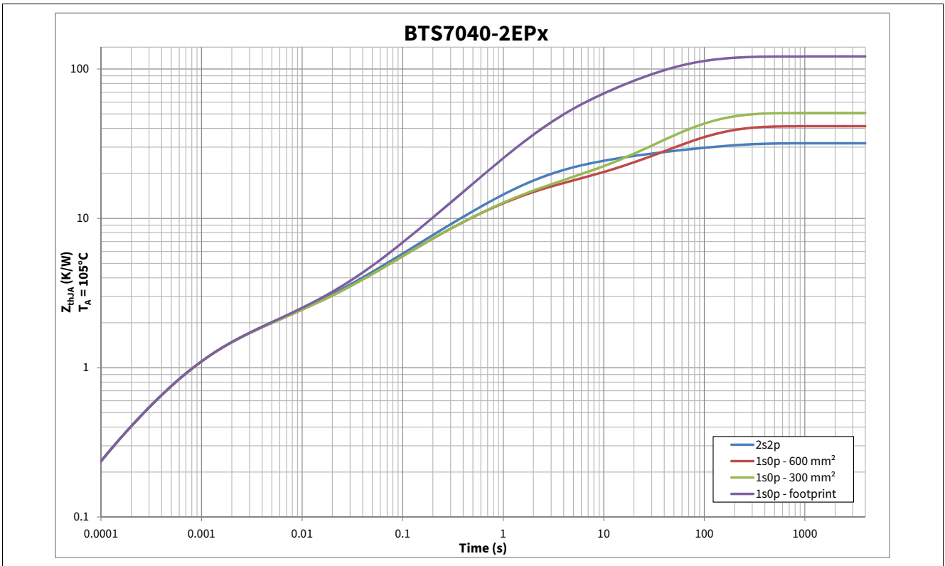
Figure 9 Typical Thermal Impedance. PCB setup according Chapter 4.4.1
