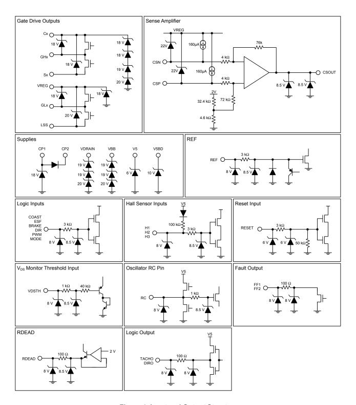
Figure 4: Input and Output Structures
