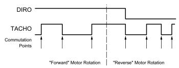
**Figure 1: Direction Indication Outputs**
