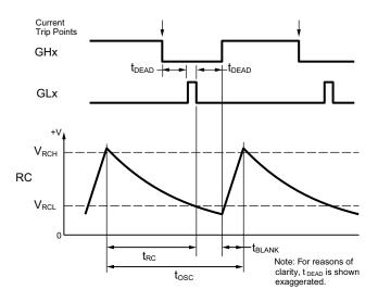
Figure 2: Internal PWM RC Timing
