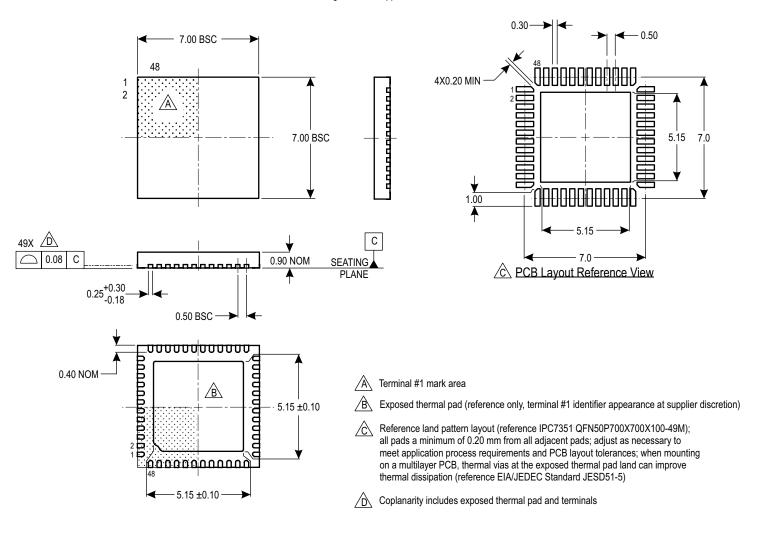
Figure 5: Package EV, 48 Terminal QFN with Exposed Thermal Pad
