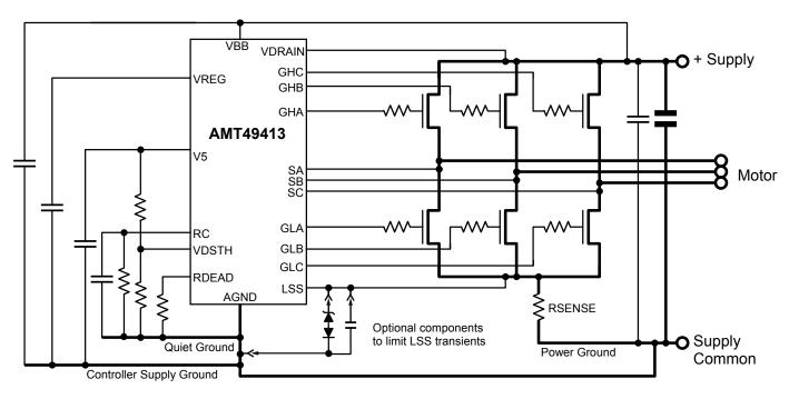
**Figure 3: Supply and Ground Connections**
