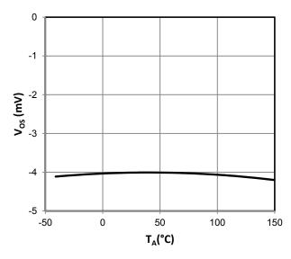
Figure 8: Uncommitted Operational Amplifier Input Offset Voltage versus Temperature
