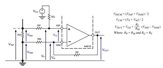
Figure 1: Operational amplifier voltage definitions
