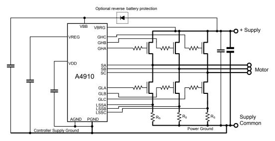
Figure 13. Supply Routing Suggestions
