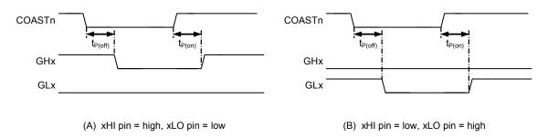
Figure 4: Gate drive timing, COASTn input
