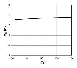
Figure 6: Current-Sense Amplifier Input Offset Voltage versus Temperature
