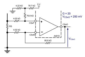
Figure 11: Typical current-sense amplifier configuration
