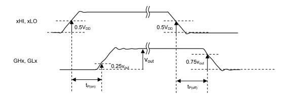
Figure 5: Propagation delay definition
