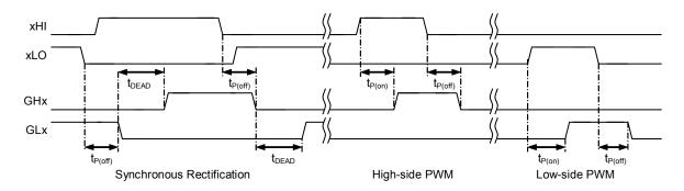
Figure 3: Gate drive timing, phase inputs
