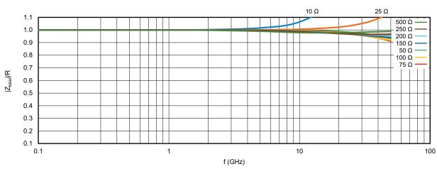
INTERNAL IMPEDANCE CURVES (|Z<sub>TOTAL</sub>| / R)
