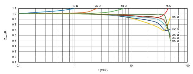
Internal impedance curve for 0603 size (N and G terminations)
