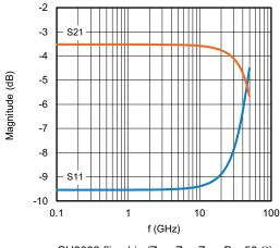
CH0603 flip chip ( $Z_0 = Z_I = Z_s = R = 50 \Omega$ )
