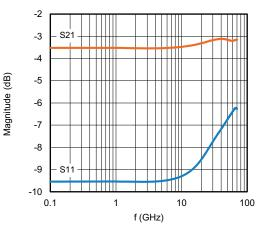
CH02016 flip chip ( $Z_0 = Z_I = Z_s = R = 100 \ \Omega$ )
