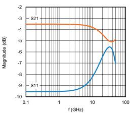
CH0603 flip chip ( $Z_0 = Z_I = Z_s = R = 100 \Omega$ )
