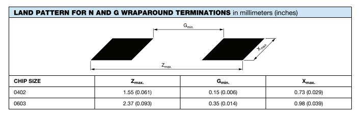
Dimension and tolerance of land pattern shall be defined by PCB designer; PCB can be designed according to IPC-7351A "Generic Requirements for Surface Mount Design and Land Pattern Standard"
