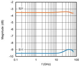
CH02016 flip chip ( $Z_0 = Z_I = Z_s = R = 50 \Omega$ )
