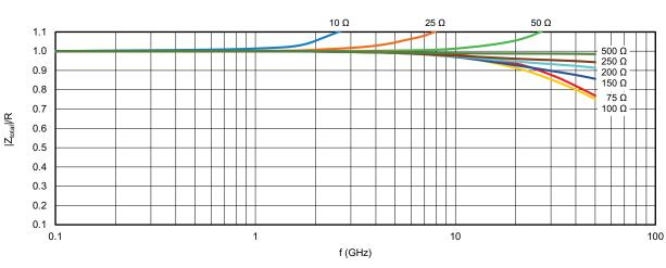
Internal impedance curve for 02016 size (F and P terminations)
