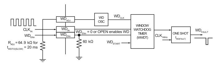
Figure 6: Watchdog Block Diagram
