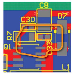
Figure 14: Boost High di/dt Loop
