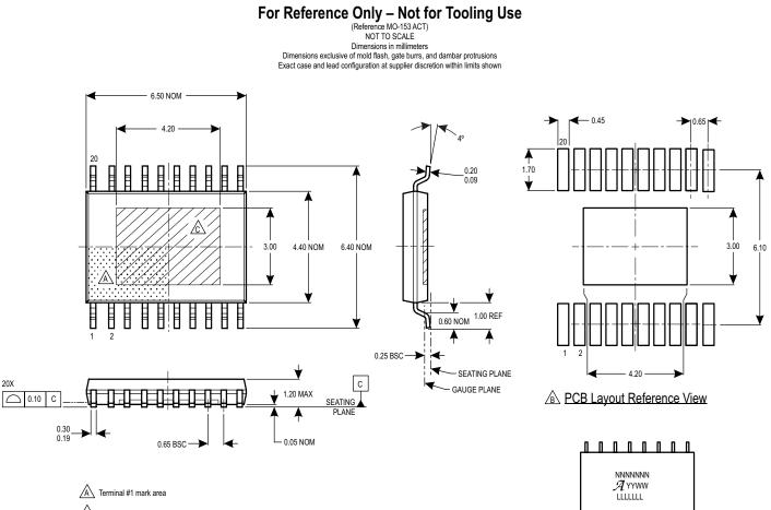
Reference land pattern layout (reference IPC7351 SOP65P640X110-21M); all pads a minimum of 0.20 mm from all adjacent pads; adjust as necessary to meet application process requirements and PCB layout tolerances; when mounting on a multilayer PCB, thermal vias at the exposed thermal pad land can improve thermal dissipation (reference EIA/JEDEC Standard JESD51-5)
