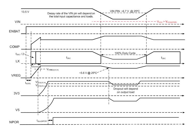
Figure 2: Input Undervoltage Timing, when VIN > V<sub>IN(STOP)</sub>
