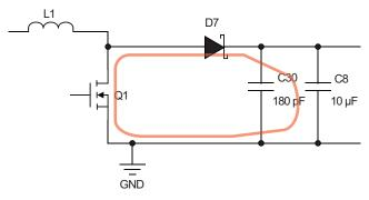
Figure 13: Boost Output Loop
