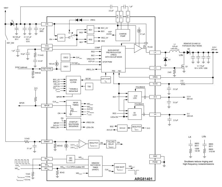
Functional Block Diagram / Typical Schematic Buck-Boost Mode (f<sub>OSC</sub> = 2 MHz)
