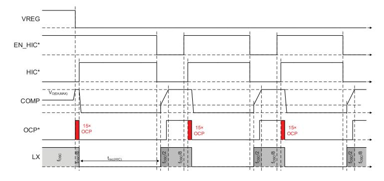
Figure 4: VREG Short Circuit to Ground Hiccup Operation
