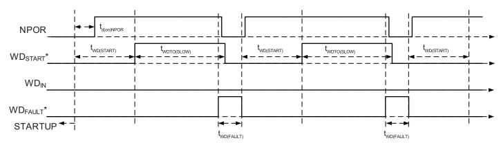
Figure 9: Window Watchdog Timer operation during slow clock fault, WD<sub>IN</sub> stuck low or high \* signal is internal to ARG81401
