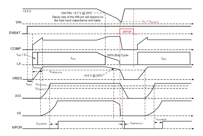
Figure 3: Input Undervoltage Timing, when VIN < V<sub>IN(STOP)</sub>
