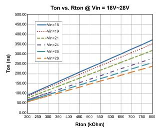
Figure 3. Ton vs. Rton Curves for AOZ2255EQI-30
