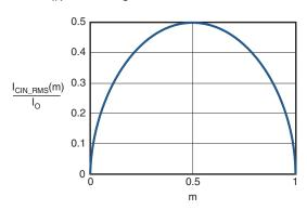
Figure 4. I<sub>CIN</sub> vs. Voltage Conversion Ratio
