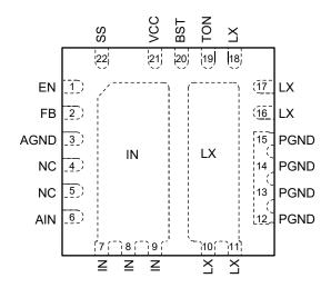
22-Pin 4mm x 4mm QFN (Top View)
