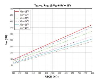
Figure 3. Ton vs. Rton Curves for AOZ2152EQI-28
