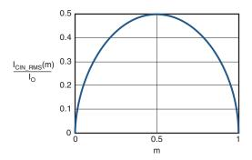
Figure 4. I<sub>CIN</sub> vs. Voltage Conversion Ratio
