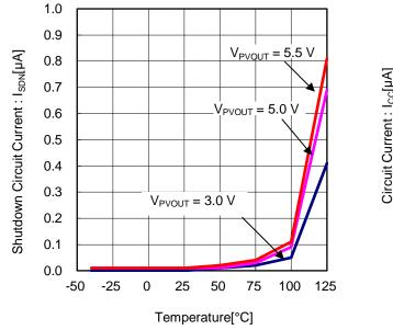
Figure 4. Shutdown Circuit Current vs Temperature
