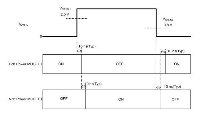
Figure 11. Control Function Timing Chart
