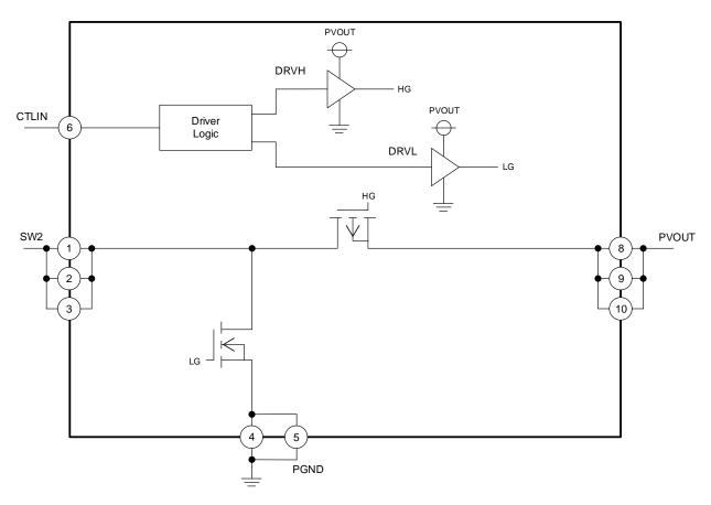
Figure 3. Block Diagram
