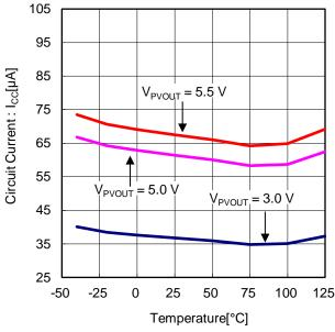
Figure 5. Circuit Current vs Temperature
