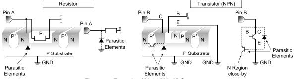
Figure 12. Example of Monolithic IC Structure
