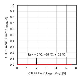
Figure 8. CTLIN Input Current vs CTLIN Pin Voltage
