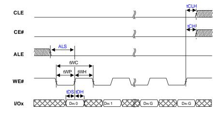
Figure 6.3 Input Data Latch Cycle
