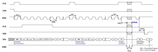
Note: tADL is the time from the WE# rising edge of final address cycle to the WE# rising edge of the first data cycle.
