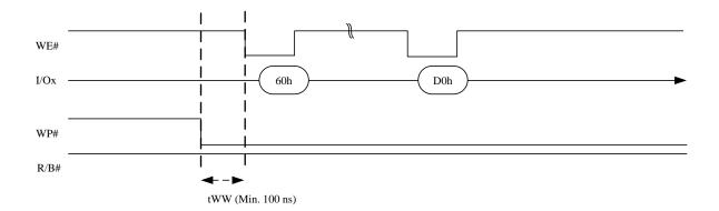
Figure 8.21 Enable/Disable Programming and Enable Erasing
