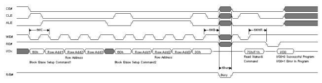
Figure 6.21 Two-Plane Block Erase Operation
