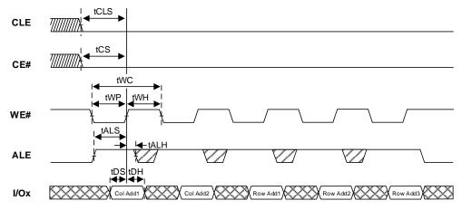
Figure 6.2 Address Latch Cycle
