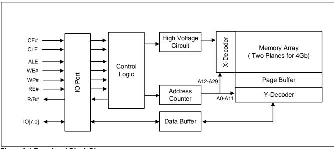
Figure 3.1 Functional Block Diagram
