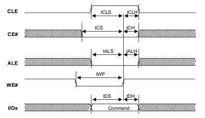
Figure 6.1 Command Latch Cycle
