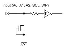
Figure 50. Input Pin Circuit Diagram
