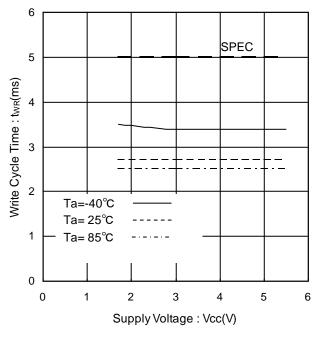
Figure 27. Write Cycle Time vs Supply Voltage
