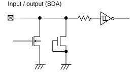
Figure 51. Input / Output Pin Circuit Diagram
