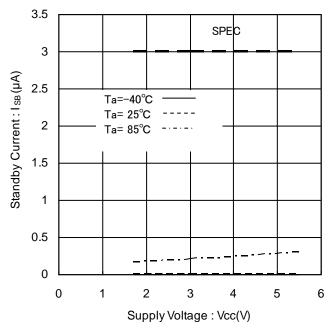
Figure 12. Standby Current vs Supply Voltage
