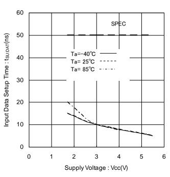
Figure 21. Input Data Setup Time vs Supply Voltage (HIGH)
