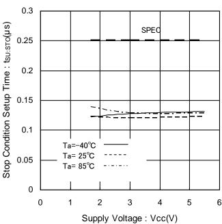
Figure 25. Stop Condition Setup Time vs Supply Voltage
