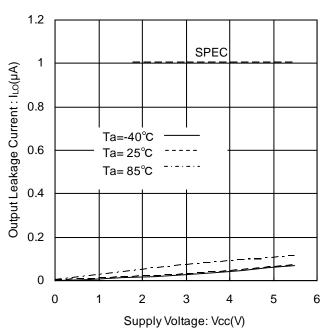
Figure 9. Output Leakage Current vs Supply Voltage (SDA)
