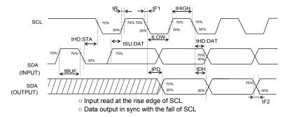
Figure 2-(a). Serial Input / Output Timing
