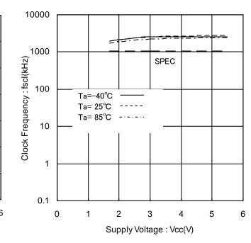
Figure 13. Clock Frequency vs Supply Voltage
