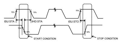
Figure 2-(b). Start-Stop Bit Timing
