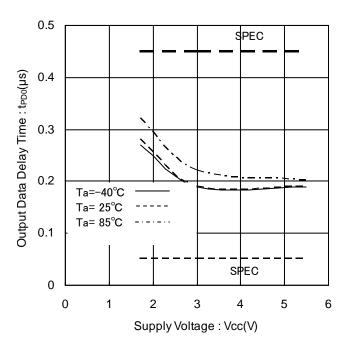
Figure 23. Output Data Delay Time vs Supply Voltage
