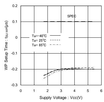
Figure 33. WP Setup Time vs Supply Voltage
