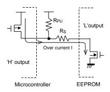
Figure 49. I/O Circuit Diagram
