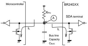
Figure.45 I/O Circuit Diagram
