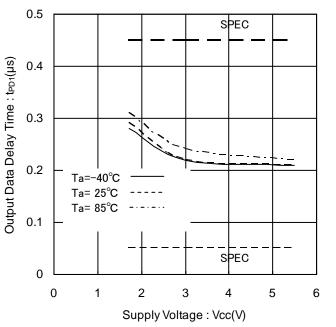
Figure 24. Output Data Delay Time vs Supply Voltage
