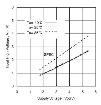
Figure 4. Input High Voltage vs Supply Voltage (A0,A1,A2,SCL,SDA,WP)
