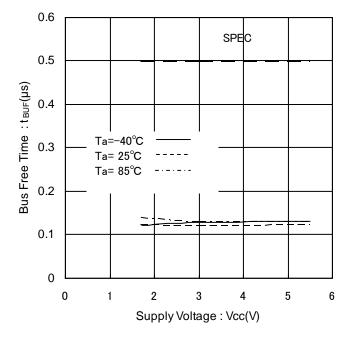
Figure 26. Bus Free Time vs Supply Voltage
