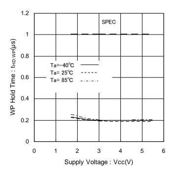
Figure 32. WP Hold Time vs Supply Voltage
