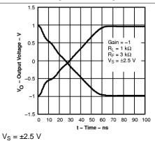
Figure 35. Settling Time
