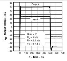
Figure 63. Small-Signal Transient Response
