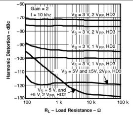
Figure 44. Harmonic Distortion vs Load Resistance
