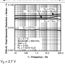
Figure 48. Total Harmonic Distortion + Noise vs Frequency
