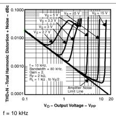
Figure 54. Total Harmonic Distortion + Noise vs Output Voltage
