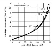
Figure 6. Negative Voltage Headroom vs Sink Current
