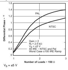
Figure 59. Differential Phase vs Number of Loads
