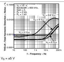
Figure 51. Total Harmonic Distortion + Noise vs Frequency
