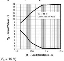
Figure 9. Output Voltage vs Load Resistance
