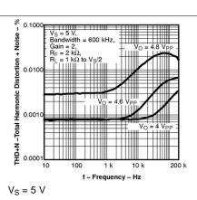
Figure 50. Total Harmonic Distortion + Noise vs Frequency
