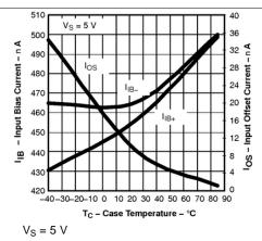
Figure 61. Input Bias and Offset Current vs Temperature
