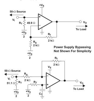
Figure 70. DC-Coupled Single Supply Operation
