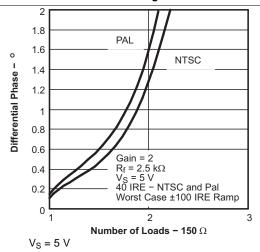
Figure 57. Differential Phase vs Number of Loads
