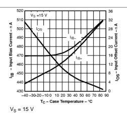
Figure 62. Input Bias and Offset Current vs Temperature
