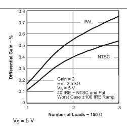
Figure 56. Differential Gain vs Number of Loads
