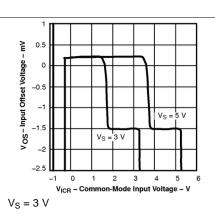
Figure 2. Input Offset Voltage vs Common-mode Input Voltage
