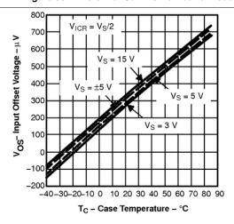
Figure 60. Input Offset Voltage vs Temperature
