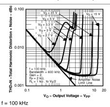
Figure 55. Total Harmonic Distortion + Noise vs Output Voltage
