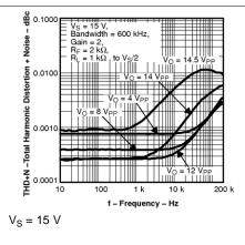
Figure 52. Total Harmonic Distortion + Noise vs Frequency
