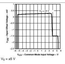
Figure 3. Input Offset Voltage vs Common-Mode Input Voltage
