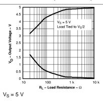
Figure 7. Output Voltage vs Load Resistance
