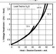
Figure 5. Positive Voltage Headroom vs Source Current
