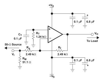
Figure 69. Wideband, Inverting Gain Configuration
