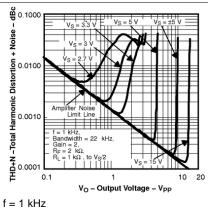
Figure 53. Total Harmonic Distortion + Noise vs Output Voltage
