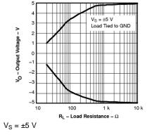
Figure 8. Output Voltage vs Load Resistance
