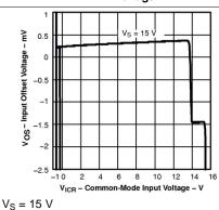
Figure 4. Input Offset Voltage vs Common-Mode Input Voltage
