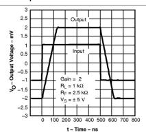
Figure 64. Large-Signal Transient Response
