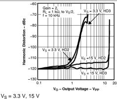
Figure 47. Harmonic Distortion vs Output Voltage
