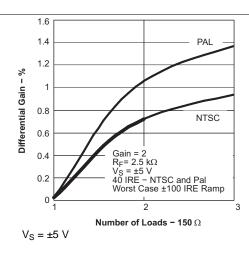
Figure 58. Differential Gain vs Number of Loads
