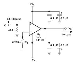
Figure 68. Wideband, Noninverting Gain Configuration
