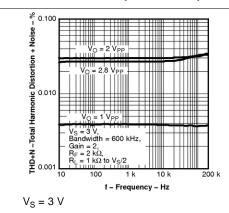
Figure 49. Total Harmonic Distortion + Noise vs Frequency
