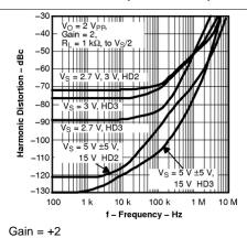
Figure 43. Harmonic Distortion vs Frequency
