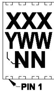
8-Lead TDFN (2x3x0.8 mm)(MCP6V17)
