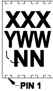
8-Lead TDFN (2 x 3 x 0.8 mm) (MCP6V37)
