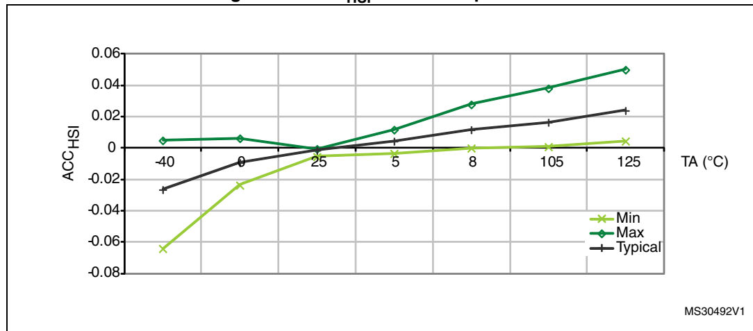
Figure 31. ACC_{HSI} versus temperature
