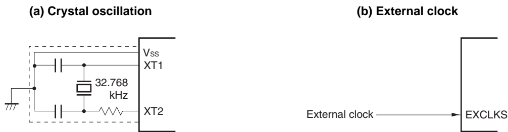
Figure 5-24. Example of External Circuit of XT1 Oscillator
