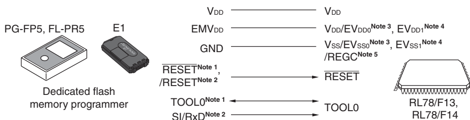
Figure 30-2. Communication with Dedicated Flash Memory Programmer
