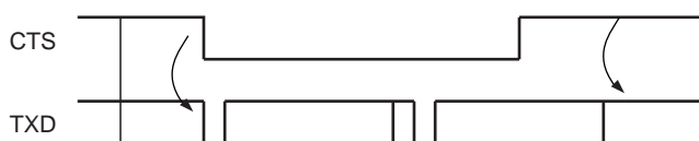
Figure 36-28. Transmitter Behavior when Operating with Hardware Handshaking
