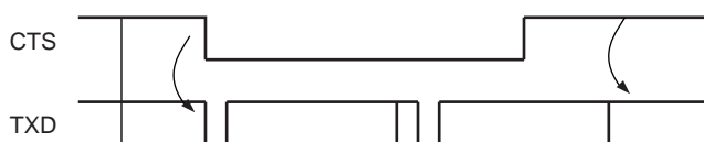
Figure 36-28. Transmitter Behavior when Operating with Hardware Handshaking
