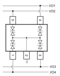
**Bidirection Protection of Four Lines**
