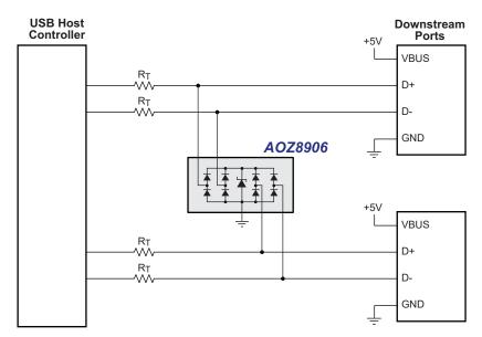
Figure 1. USB High Speed Ports
