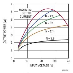
Figure 2. Output Power for 5V Output
