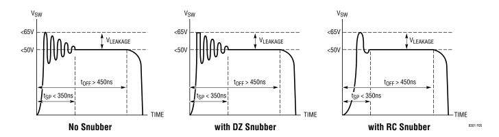
Figure 5. Maximum Voltages for SW Pin Flyback Waveform
