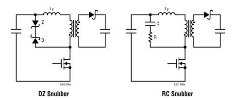
Figure 6. Snubber Circuits
