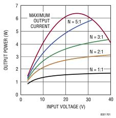
Figure 1. Output Power for 3.3V Output
