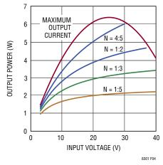
Figure 4. Output Power for 24V Output
