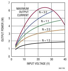
Figure 3. Output Power for 12V Output
