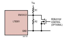
Figure 7. Undervoltage Lockout (UVLO)
