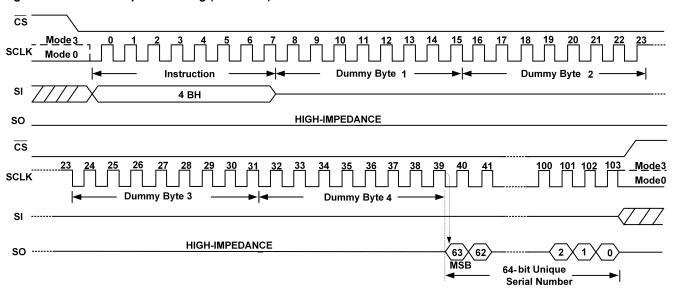
Figure 10-1. Read Unique ID Timing (SPI Mode)
