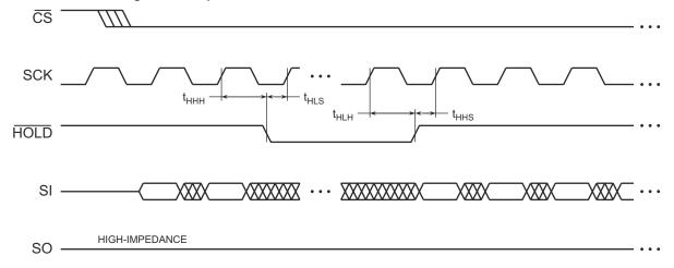
Figure 14-5. HOLD Timing – Serial Output
