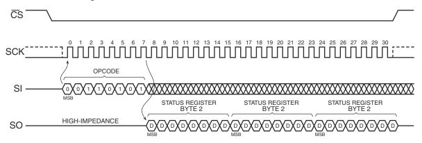
Table 11-3 shows the bit assignments for Status Register 3. This register can be read using the Status Register 3 Read command (15h), and written using the Status Register 3 Write command (11h).
