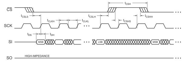
Figure 14-2. Serial Output Timing
