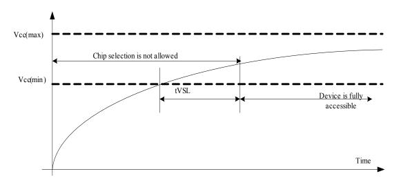
Figure 13-1. Power-up Timing and Voltage Levels
