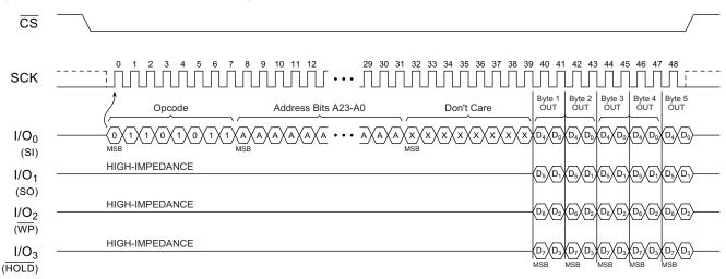
Figure 7-6. Quad-Output Fast Read Array
