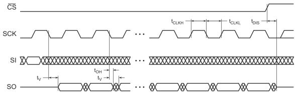
Figure 14-3. WP Timing for Write Status Register Command When BPL = 1
