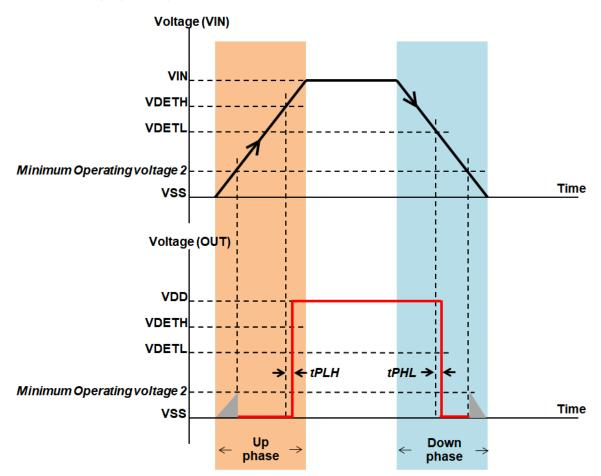
Figure 4. Voltage detection function, VIN is controlled separately from VDD, POL= "L"
