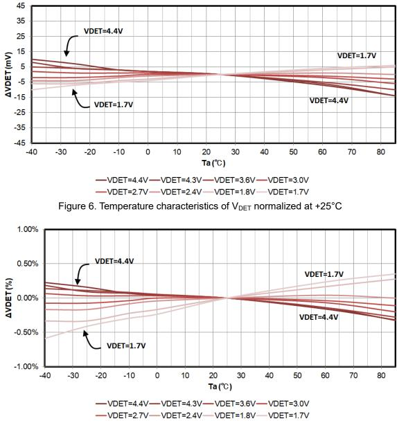
Figure 7. Temperature characteristics of  $V_{DET}$  normalized at +25°C
