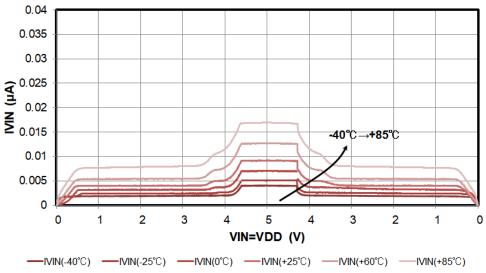
Figure 12. IVIN vs Temperature at VDETH=4.4V, VDETL=4.3V (VIN=VDD sweep), POL = "L"
