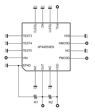
Figure 5. Reference Circuit for measurement
