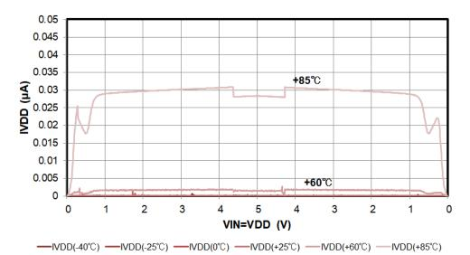
Figure 14. IVDD vs Temperature at VDETH=4.4V, VDETL=4.3V (VIN=VDD sweep), POL = "L"
