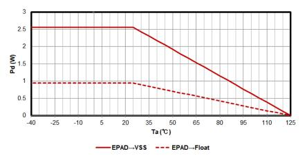
Figure 2. Power Dissipation vs Temperature
