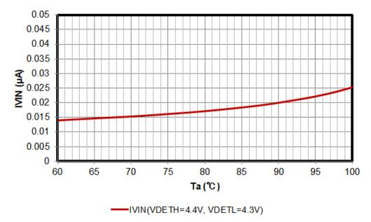
Figure 13. IVIN vs Temperature at VIN=VDD=5.5V, POL = "L"
