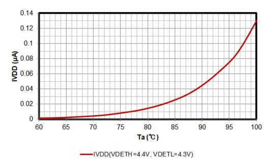
Figure 15. IVDD vs Temperature at VIN=VDD=5.5V, POL= "L"
