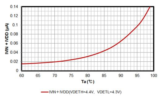
Figure 16. IVIN+IVDD vs Temperature
