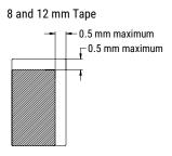
Figure 4 - Bending Radius
