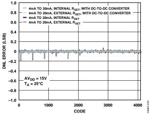
Figure 10. Differential Nonlinearity Error vs. DAC Code
