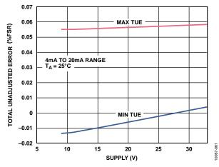
Figure 22. Total Unadjusted Error vs. Supply, Internal R<sub>SET</sub>
