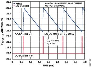
Figure 57. Operation on Reaching V<sub>MAX</sub>
