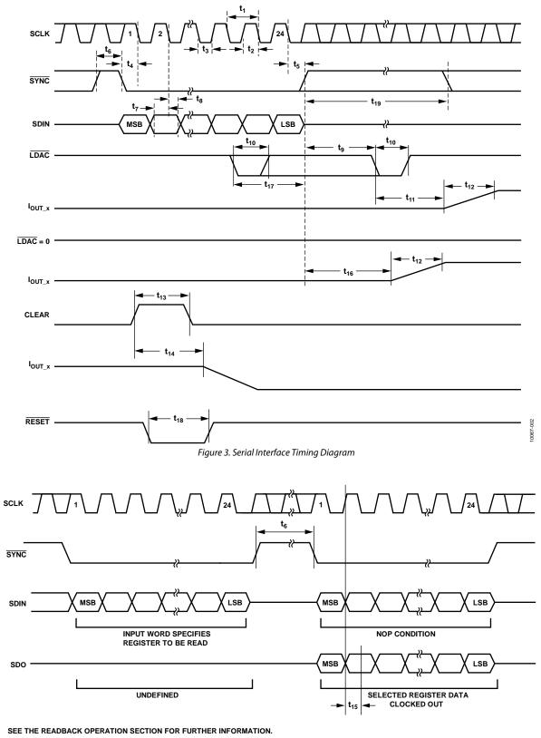
Figure 4. Readback Timing Diagram (Packet Error Checking Disabled)
