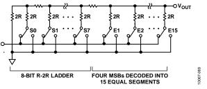
Figure 48. DAC Ladder Structure
