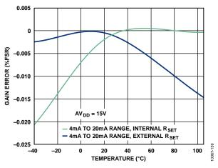
Figure 17. Gain Error vs. Temperature
