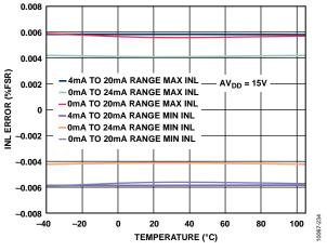
Figure 12. Integral Nonlinearity Error vs. Temperature, Internal RSET
