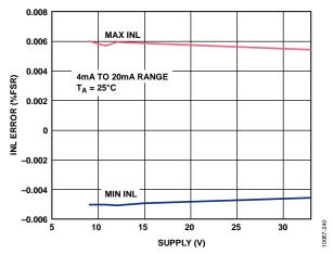
Figure 18. Integral Nonlinearity Error vs. Supply, External R<sub>SET</sub>
