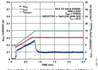
Figure 60. Alcc Current vs. Time for 24 mA Step Through 500  $\Omega$  Load with External 51 k $\Omega$  Compensation Resistor
