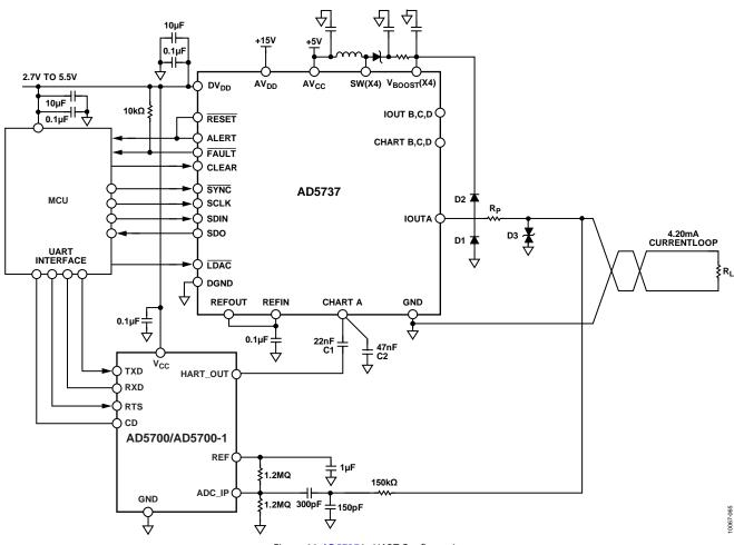
Figure 66. AD5737 in HART Configuration
