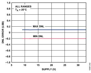
Figure 20. Differential Nonlinearity Error vs. Supply
