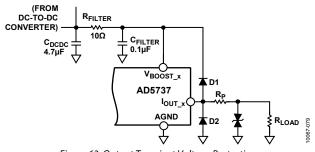
Figure 63. Output Transient Voltage Protection
