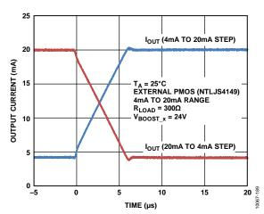
Figure 29. Output Current Settling Time with External PMOS Transistor
