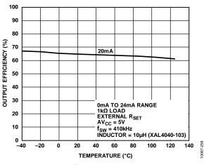
Figure 36. Output Efficiency vs. Temperature (See Figure 56)
