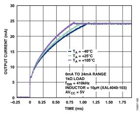
Figure 27. Output Current Settling Time with DC-to-DC Converter over Temperature (See Figure 56)
