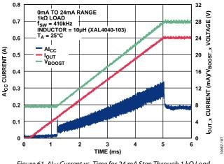
Figure 61. Alcc Current vs. Time for 24 mA Step Through 1 k $\Omega$  Load with Slew Rate Control
