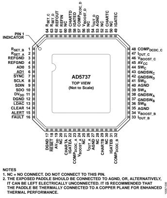
Figure 8. Pin Configuration
