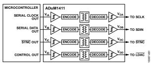
Figure 65. 4-Channel Isolated Interface to the AD5737
