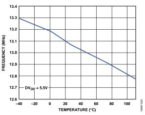
Figure 46. Internal Oscillator Frequency vs. Temperature
