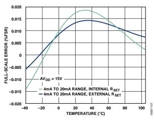
Figure 16. Full-Scale Error vs. Temperature
