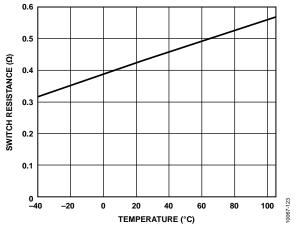
Figure 37. Switch Resistance vs. Temperature
