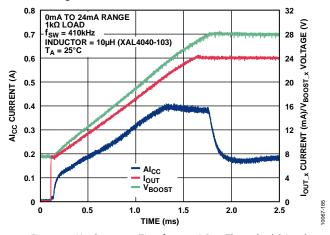
Figure 59. Al<sub>CC</sub> Current vs. Time for 24 mA Step Through 1 k $\Omega$  Load with External 51 k $\Omega$  Compensation Resistor
