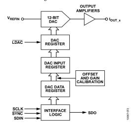
Figure 50. Simplified Serial Interface of the Input Loading Circuitry for One DAC Channel
