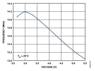
Figure 47. Internal Oscillator Frequency vs. DV<sub>DD</sub> Supply Voltage
