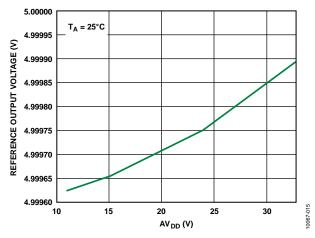
Figure 43. REFOUT Voltage vs. AVDD
