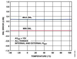
Figure 14. Differential Nonlinearity Error vs. Temperature
