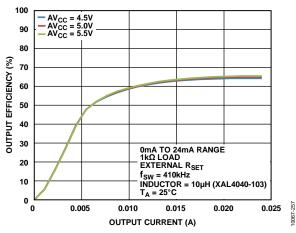
Figure 35. Output Efficiency vs. Output Current (See Figure 56)
