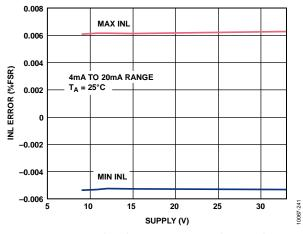
Figure 19. Integral Nonlinearity Error vs. Supply, Internal R<sub>SET</sub>
