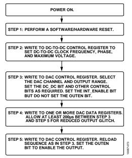
Figure 51. Programming Sequence to Correctly Enable the Output
