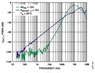
Figure 32. IOUT\_x PSRR vs. Frequency
