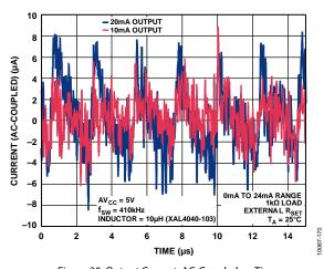
Figure 30. Output Current, AC-Coupled vs. Time with DC-to-DC Converter (See Figure 56)
