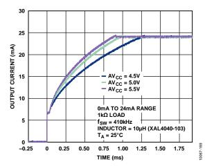
Figure 28. Output Current Settling Time with DC-to-DC Converter over AVcc (See Figure 56)
