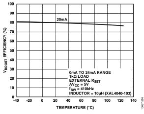
Figure 34. Efficiency at V<sub>BOOST\_x</sub> vs. Temperature (See Figure 56)
