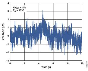
Figure 39. REFOUT Output Noise (0.1 Hz to 10 Hz Bandwidth)
