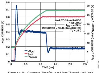
Figure 58. Alcc Current vs. Time for 24 mA Step Through 1 k $\Omega$  Load with Internal Compensation Resistor
