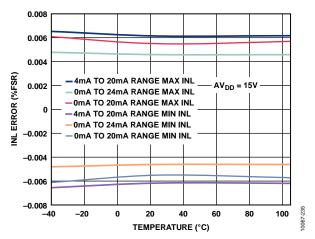
Figure 13. Integral Nonlinearity Error vs. Temperature, External RSET
