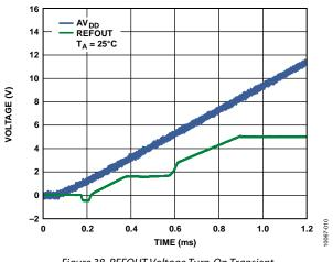
Figure 38. REFOUT Voltage Turn-On Transient
