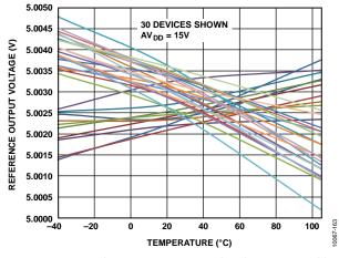
Figure 41. REFOUT Voltage vs. Temperature (When the AD5737 is soldered onto a PCB, the reference shifts due to thermal shock on the package. The average output voltage shift is –4 mV. Measurement of these parts after seven days shows that the outputs typically shift back 2 mV toward their initial values. This second shift is due to the relaxation of stress incurred during soldering.)
