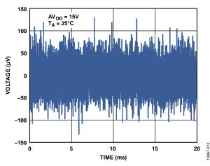
Figure 40. REFOUT Output Noise (100 kHz Bandwidth)
