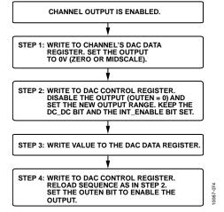
Figure 52. Programming Sequence to Change the Output Range
