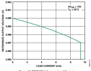
Figure 42. REFOUT Voltage vs. Load Current
