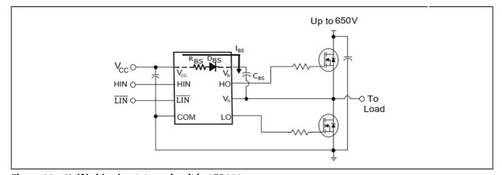
Figure 16 Half bridge bootstrap circuit in 2ED210x
