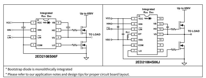
Figure 1 Typical application block diagram
