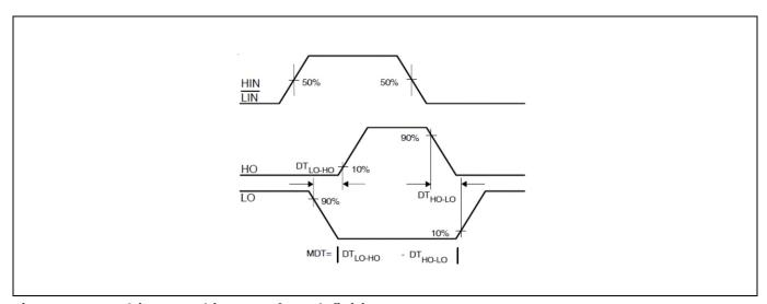
Figure 8 Deadtime matching waveform definition
