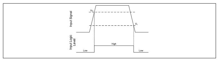
Figure 12 HIN & /LIN input thresholds
