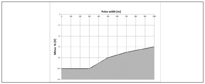
Figure 21 Negative VS transient SOA for 2ED2108 (4) S06F (J) @ VBS=15 V
