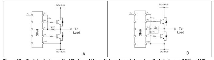
Figure 25 Resistor between the VS pin and the switch node and clamping diode between COM and VS
