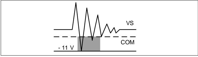
Figure 22 Headroom for HV level shifter data transmission
