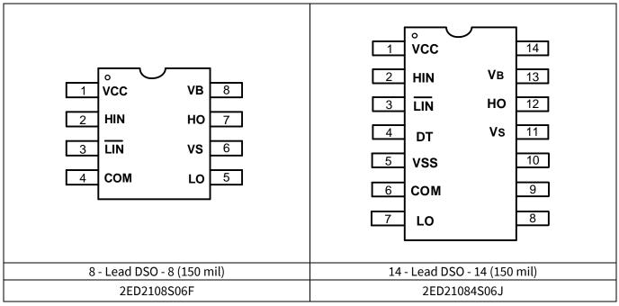
Figure 3 2ED2108 (4) S06 F(J) pin assignments (top view)
