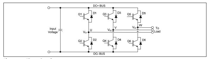
Figure 18 Three phase inverter
