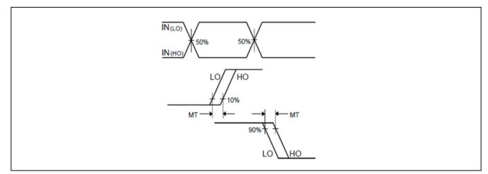
Figure 11 Delay matching waveform definition
