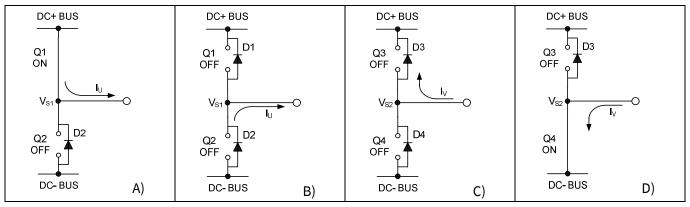
Figure 19 A) Q1 conducting
