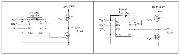
Figure 14 2ED210x with integrated components
