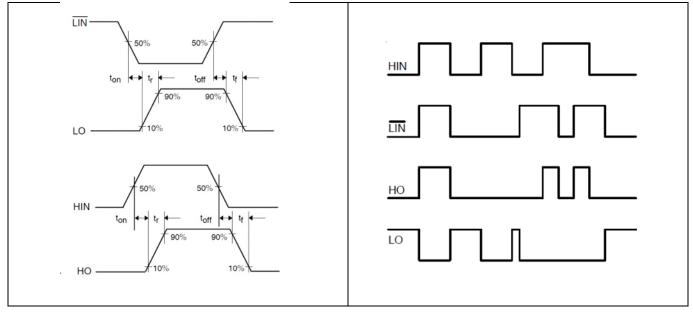
Figure 6 Switching timing diagram
