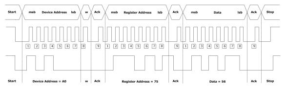
Figure 11 • Read Cycle Diagram
