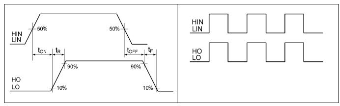
Figure 6 Switching timing diagram
