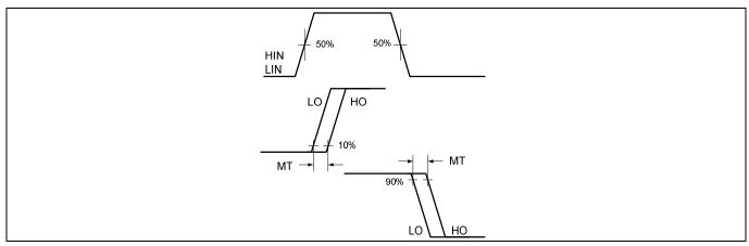
Figure 8 Delay matching waveform definition
