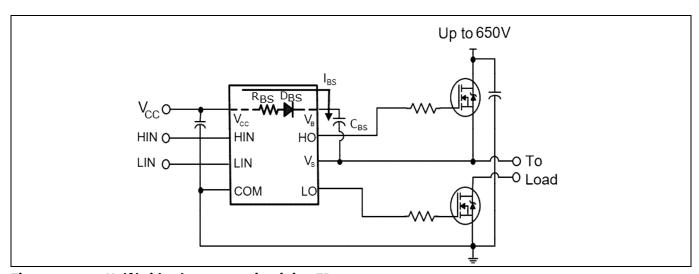
Figure 13 Half bridge bootstrap circuit in 2ED218x
