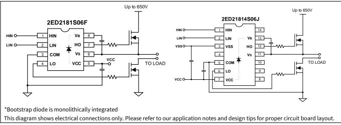
Figure 1 Typical application block diagram
