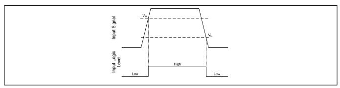
Figure 9 HIN & LIN input thresholds
