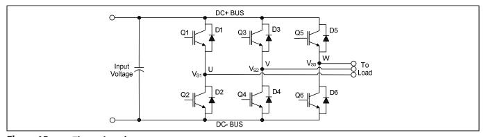
Figure 15 Three phase inverter
