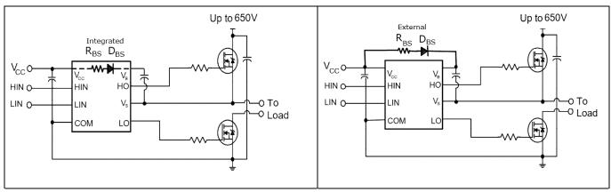
Figure 11 2ED218x with integrated components Figure 12 Standard bootstrap gate driver
