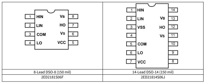
Figure 3 2ED2181(4)S06F(J) pin assignments (top view)
