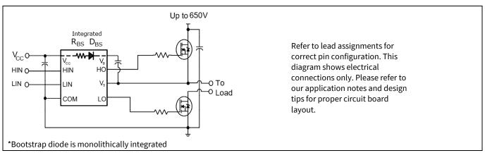
Figure 1 Typical application block diagram
