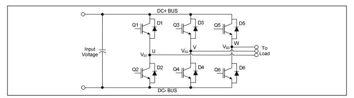
Figure 15 Three phase inverter
