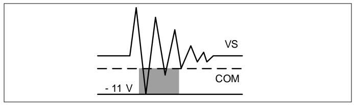
Figure 19 Headroom for HV level shifter data transmission
