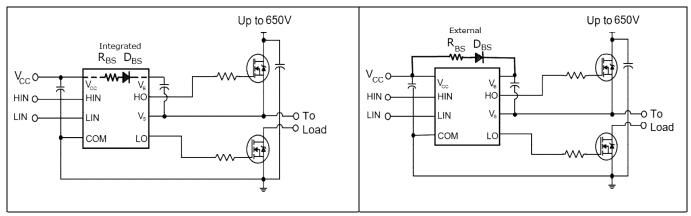
Figure 11 2ED210x with integrated components Figure 12 Standard bootstrap gate driver
