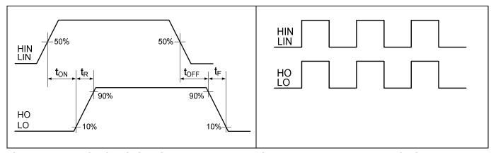
Figure 6 Switching timing diagram
