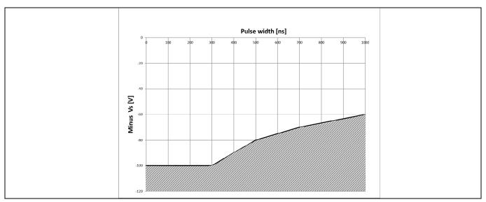
Figure 18 Negative VS transient SOA for 2ED2106 (4) S06F (J) @ VBS = 15 V
