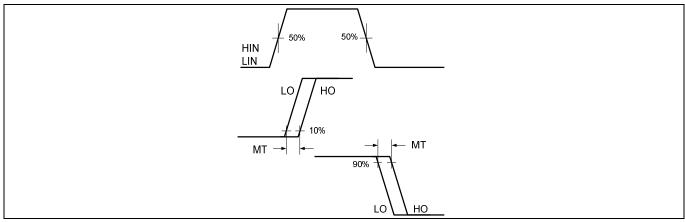
Figure 8 Delay matching waveform definition
