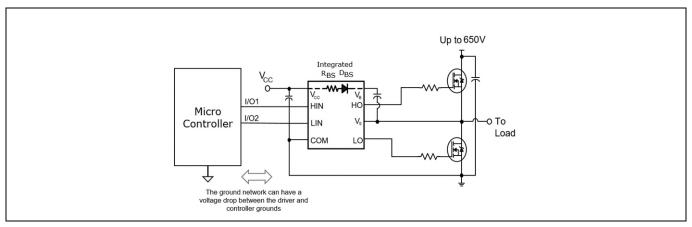
Figure 14 Negative voltage tolerance on inputs of upto -5 V
