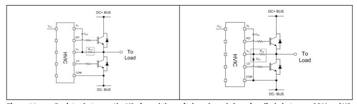
Figure 22 Resistor between the VS pin and the switch node and clamping diode between COM and VS
