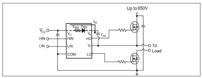
Figure 13 Half bridge bootstrap circuit in 2ED210x
