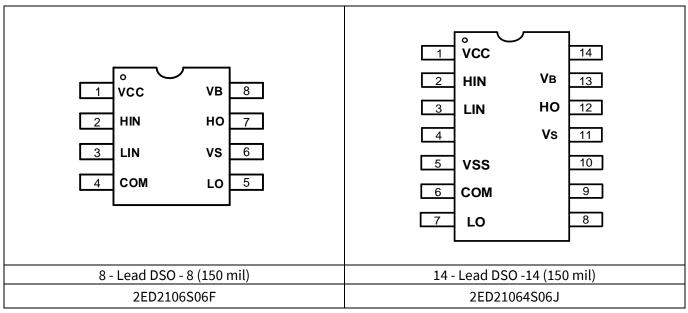
Figure 3 2ED2106(4)S06F(J) pin assignments (top view)
