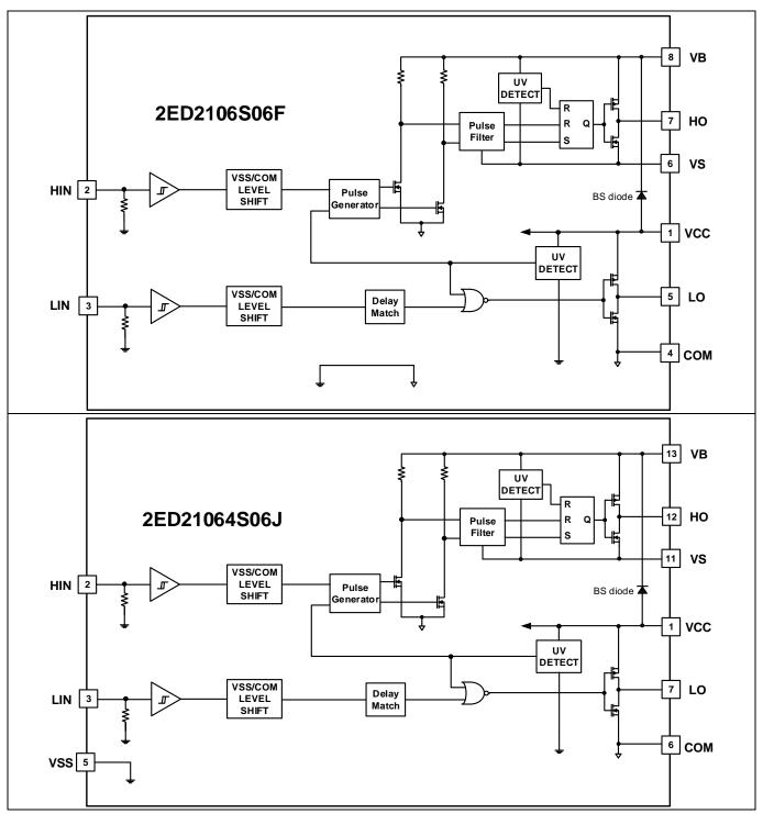
Figure 2 Block diagrams
