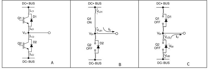
Figure 17 Figure A shows the parasitic elements. Figure B shows the generation of V<sub>s</sub> positive. Figure C shows the generation of V<sub>s</sub> negative
