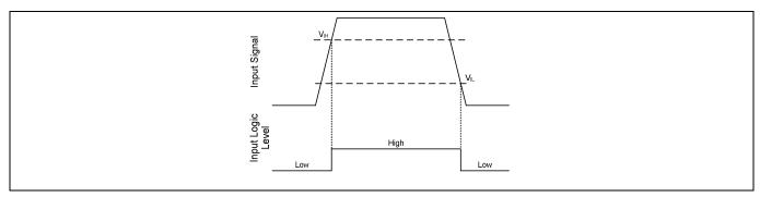
Figure 9 HIN & LIN input thresholds
