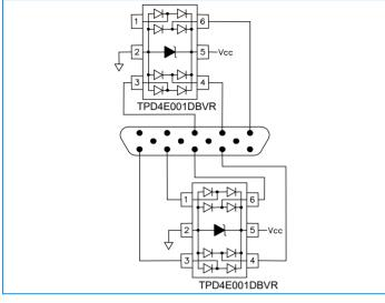
Figure 5 - Dual USB Port Protection
