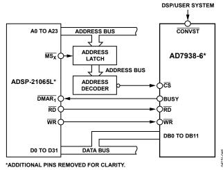
Figure 44. Interfacing to the ADSP-21065L
