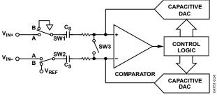
Figure 16. ADC Conversion Phase
