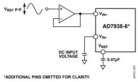
Figure 30. Pseudo Differential Mode Connection Diagram
