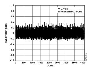
Figure 8. AD7938-6 Typical DNL at  $V_{DD} = 5 V$
