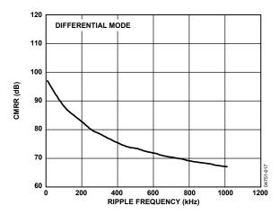
Figure 14. CMRR vs. Input Frequency with  $V_{\rm DD} = 5 \, V$  and  $3 \, V$
