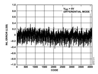
Figure 9. AD7938-6 Typical INL at  $V_{DD} = 5 V$
