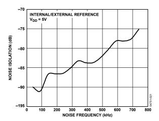
Figure 5. AD7938-6 Channel-to-Channel Isolation
