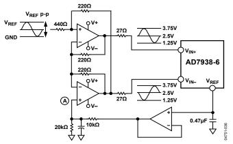
Figure 29. Dual Op Amp Circuit to Convert a Single-Ended Unipolar Signal into a Differential Signal
