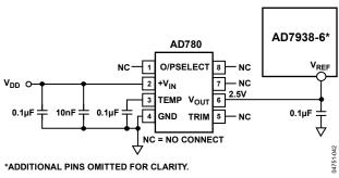
Figure 35. Typical V<sub>REF</sub> Connection Diagram
