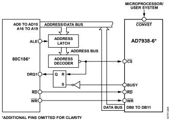
Figure 46. Interfacing to the 80C186
