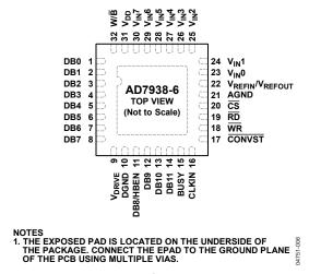
Figure 2. Pin Configuration (CP-32-7)
