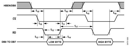
Figure 37. AD7938-6 Parallel Interface—Read Cycle Timing for Byte Mode Operation ( $W/\overline{B} = 0$ )
