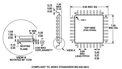
Figure 48. 32-Lead Thin Plastic Quad Flat Package [TQFP] (SU-32-2)
