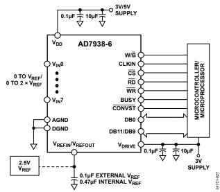
Figure 19. Typical Connection Diagram
