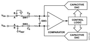
Figure 15. ADC Acquisition Phase
