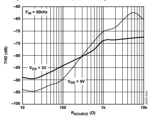
Figure 22. THD vs. Source Impedance in Differential Mode
