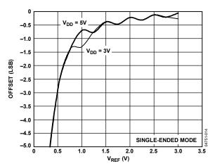
Figure 12. AD7938-6 Offset vs. V<sub>REF</sub>
