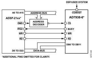
Figure 43. Interfacing to the ADSP-21xx
