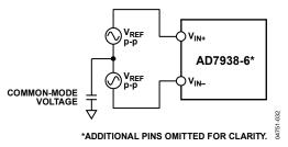
Figure 25. Differential Input Definition
