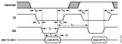
Figure 39. AD7938-6 Parallel Interface—Write Cycle Timing for Byte Mode Operation ( $W/\overline{B} = 0$ )
