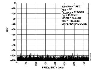
Figure 7. AD7938-6 FFT at  $V_{DD} = 5 V$
