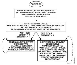
Figure 32. Programmable Sequence Flow Chart
