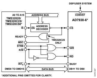
Figure 45. Interfacing to the TMS32020/TMS320C25/TMS320C5x
