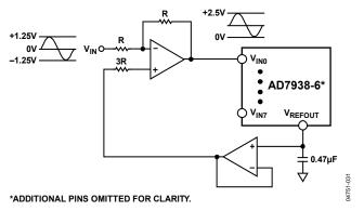
Figure 24. Single-Ended Mode Connection Diagram
