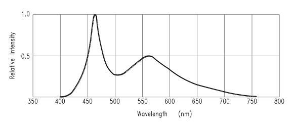
Fig.1 RELATIVE INTENSITY VS. WAVELENGTH
