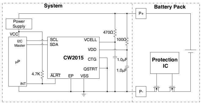
Figure 1. Typical Application Diagram (System Side)
