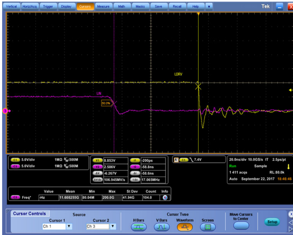
Figure 31. Low Side Turn-Off Propagation Delay (NCP51530A)
