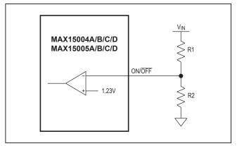
Figure 1. Setting the MAX15004A/B/MAX15005A/B Undervoltage-Lockout Threshold
