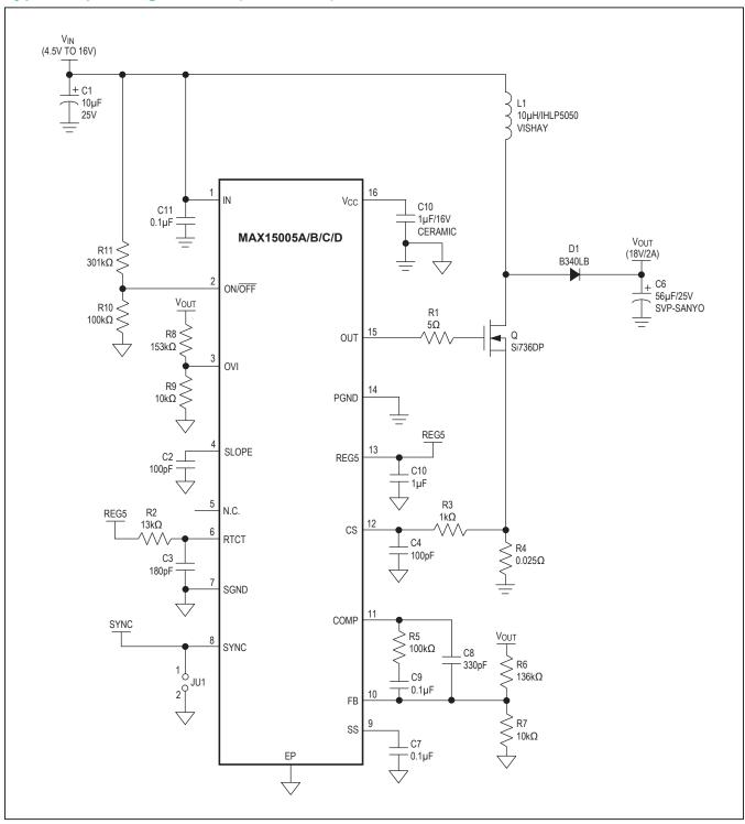
Figure 8. Boost Application Circuit
