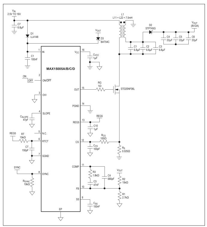
Figure 6. SEPIC Application Circuit
