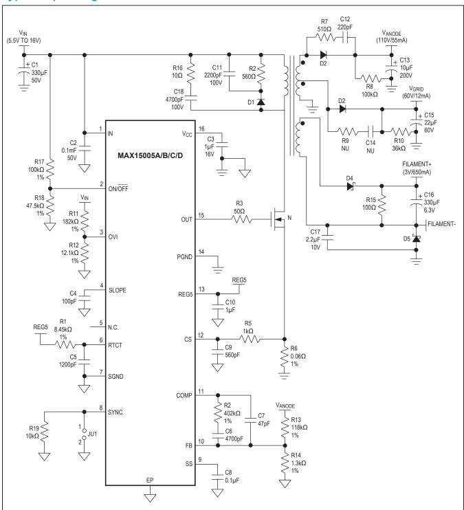
Figure 7. VFD Flyback Application Circuit
