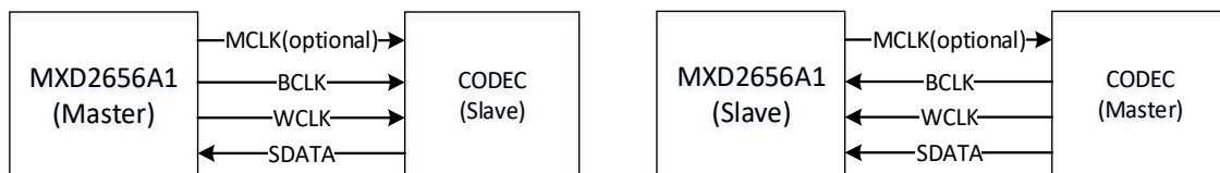
Figure 36 I2S interface signals
