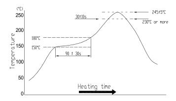
Temperature profile for reflow soldering
