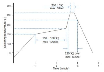
Recommended IR Reflow Soldering Profile
