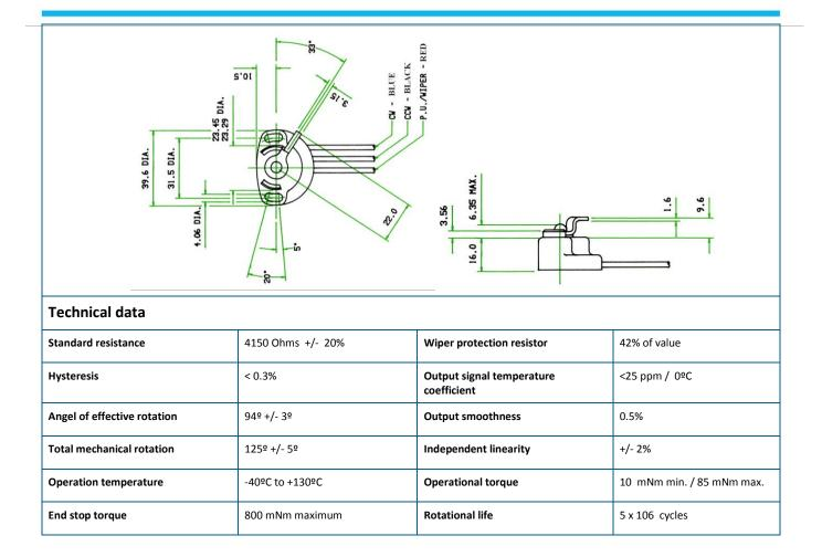
Conductive polymer potentiometer for automotive and other similar demanding applications. A high performance cost effective potentiometer, with long endurance life and protection from engine compartment environment. Termination via 280 mm long flying leads.
