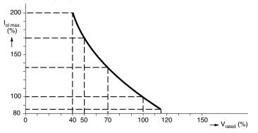
I<sub>ol max.</sub> as stated in the electrical data and ordering information tables, is the maximum overload current that may flow through the PTC when passing from the low ohmic to high ohmic state at rated voltage.
