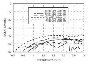
Isolation When VL is Connected to OP1\*
