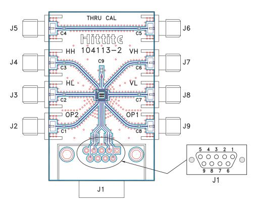
The circuit board used in the final application should be generated with proper RF circuit design techniques. Signal lines at the RF port should have 50 ohm impedance and the package ground leads and exposed paddle should be connected directly to the ground plane similar to that shown above. A generous number of ground vias should be used to interconnect top/bottom ground planes. The evaluation circuit board shown above is available from Hittite Microwave Corporation upon request.
