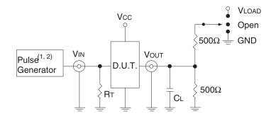
Test Circuits for All Outputs
