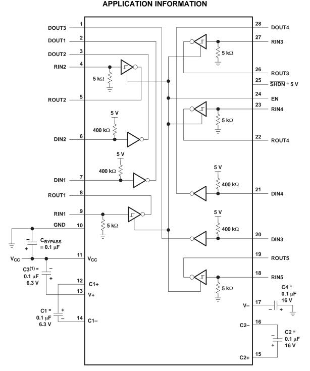
(1) C3 can be connected to  $V_{\mbox{CC}}$  or GND.
