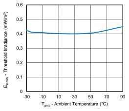
Fig. 6 - Sensitivity vs. Ambient Temperature
