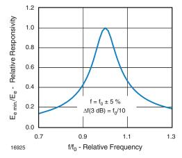
Fig. 5 - Frequency Dependence of Responsivity
