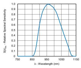
Fig. 7 - Relative Spectral Sensitivity vs. Wavelength
