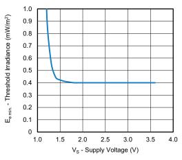
Fig. 9 - Sensitivity vs. Supply Voltage
