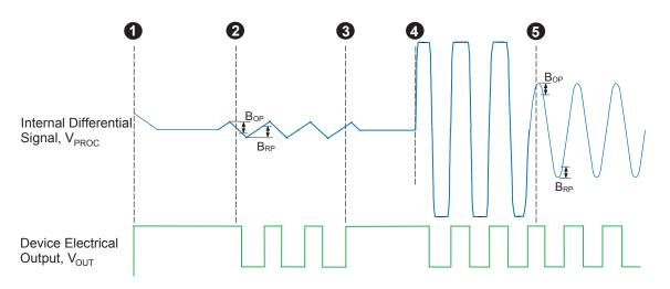
Figure 7: Operation of Running Mode Gain Adjust
