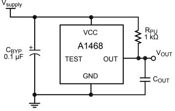
Figure 6: Typical Application Diagram
