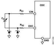
Figure 48. AD7150 CIN Overvoltage Protection
