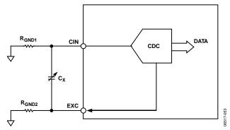
Figure 45. Parasitic Resistance to Ground
