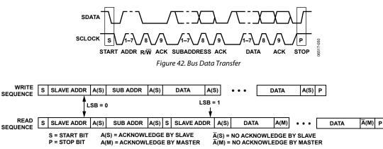
Figure 43. Write and Read Sequences
