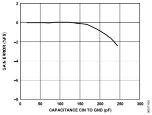
Figure 5. Capacitance Input Gain Error vs. Capacitance CIN to GND,  $V_{\rm DD}$  = 3.3 V, CIN to EXC = 2 pF
