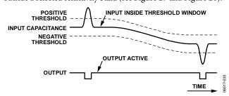
Figure 27. In-Window (Adaptive) Threshold Mode
