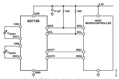
Figure 52. AD7150 Interfaced to a Host Microcontroller
