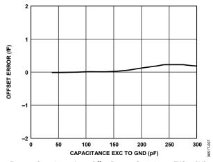
Figure 7. Capacitance Input Offset Error vs. Capacitance EXC to GND,  $V_{DD} = 3.3 \ V$ , CIN Pin Open Circuit
