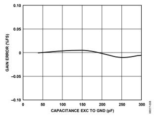
Figure 8. Capacitance Input Gain Error vs. Capacitance EXC to GND,  $V_{\rm DD}$  = 3.3 V, CIN to EXC = 2 pF
