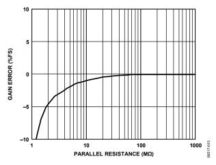
Figure 15. Capacitance Input Gain Error vs. Parallel Resistance,  $V_{\rm DD}=3.3~V, {\it CIN}$  to EXC = 2 pF
