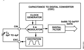
Figure 23. CDC Simplified Block Diagram
