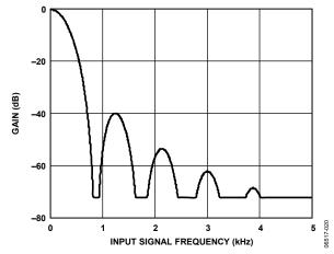
Figure 20. Capacitance Channel Frequency Response
