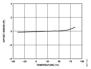
Figure 16. Capacitance Input Offset Error vs. Temperature,  $V_{\rm DD}$  = 3.3 V, CIN and EXC Pins Open Circuit
