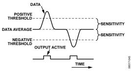
Figure 37. Threshold Sensitivity
