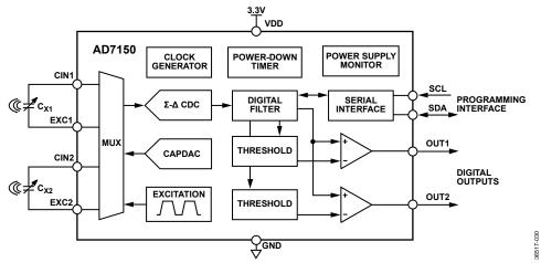
Figure 22. AD7150 Block Diagram
