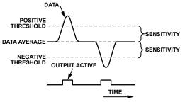
Figure 31. Threshold Sensitivity
