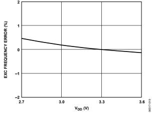
Figure 19. EXC Frequency Error vs.  $V_{\text{DD}}$
