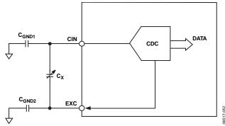
Figure 44. Parasitic Capacitance to Ground
