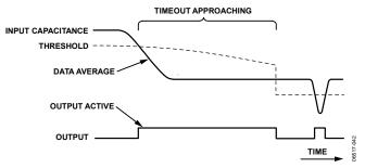
Figure 34. Approaching Timeout in Negative Threshold Mode Shortens False Output Trigger
