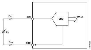
Figure 47. Parasitic Serial Resistance
