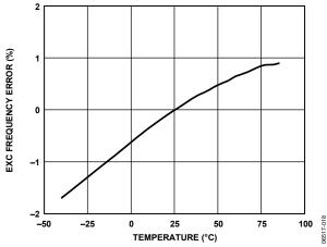
Figure 18. EXC Frequency Error vs. Temperature,  $V_{\text{DD}} = 3.3 \ V$
