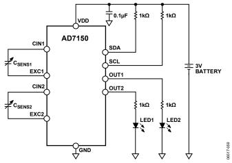
Figure 51. AD7150 Standalone Operation Application Diagram
