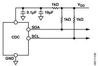
Figure 50. AD7150 V<sub>DD</sub> Decoupling and Filtering
