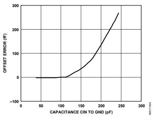
Figure 4. Capacitance Input Offset Error vs. Capacitance CIN to GND,  $V_{\rm DD}=3.3$  V, EXC Pin Open Circuit
