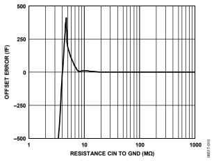
Figure 10. Capacitance Input Offset Error vs. Resistance CIN to GND,  $V_{\rm DD}=3.3$  V, EXC Pin Open Circuit
