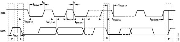
Figure 2. Serial Interface Timing Diagram
