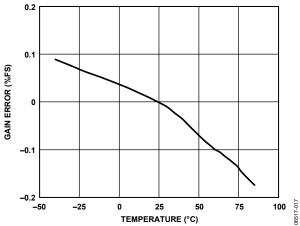
Figure 17. Capacitance Input Gain Error vs. Temperature,  $V_{\rm DD}$  = 3.3 V, CIN to EXC = 2 pF
