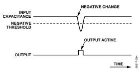
Figure 26. Negative Threshold Mode Indicates Negative Change in Input Capacitance
