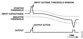
Figure 28. Out-Window (Adaptive) Threshold Mode
