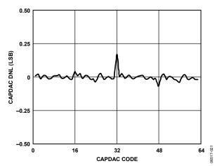
Figure 21. CAPDAC Differential Nonlinearity (DNL),  $V_{DD} = 3.3 \text{ V}$
