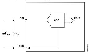
Figure 46. Parasitic Parallel Resistance
