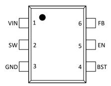
Figure 6-1. 6-Pin SOT563 DRL Package (Top View)
