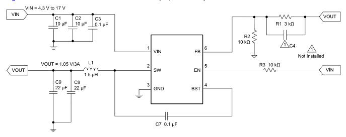
Figure 9-1. TPS563207S 1.05-V/3-A Reference Design
