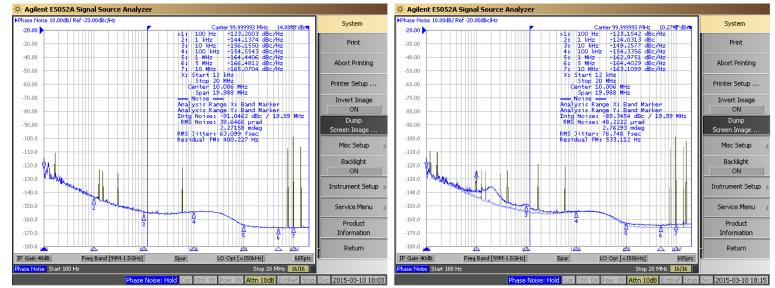
Figure 1. 524S Reference Phase Noise 63fs (12kHz to 20MHz)
