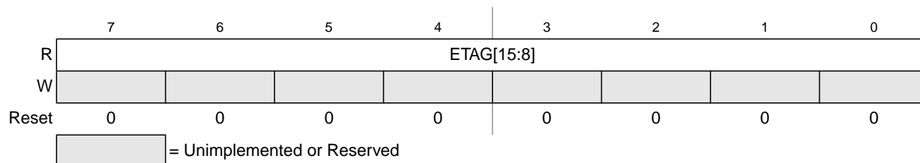
Figure 4-18. EEE Tag Counter High Register (ETAGHI)
