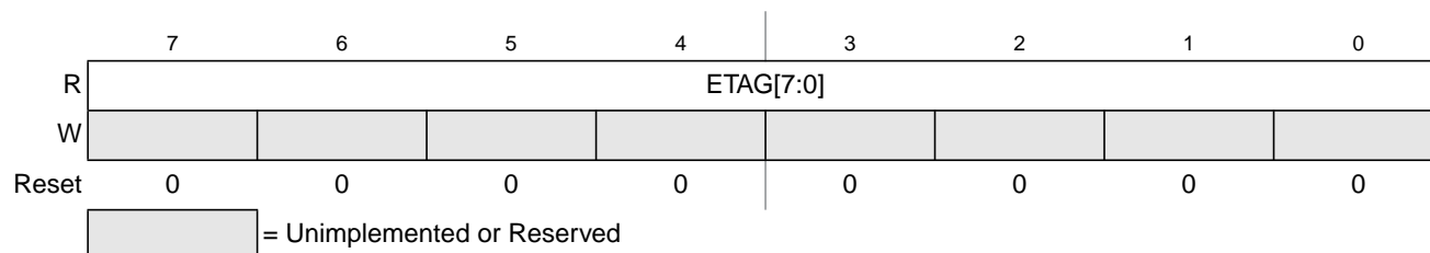
Figure 10-19. EEE Tag Counter Low Register (ETAGLO)
