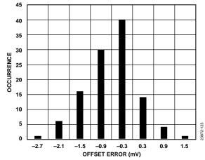
Figure 16. Offset Error Distribution Histogram
