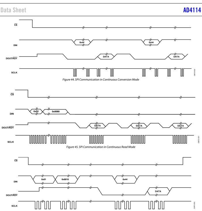
Figure 46. SPI Communication in Single Conversion Mode
