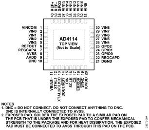
Figure 4. Pin Configuration
