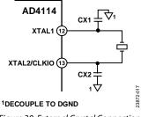
Figure 30. External Crystal Connections
