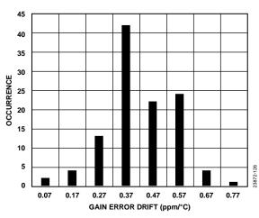
Figure 19. Gain Error Drift Distribution Histogram
