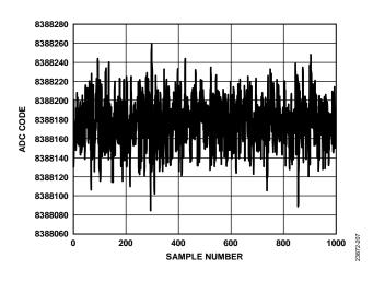
Figure 7. Noise (Output Data Rate = 31.25 kSPS)
