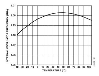
Figure 14. Internal Oscillator Frequency vs. Temperature
