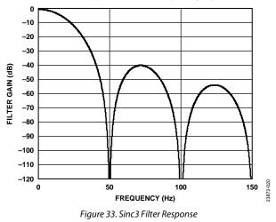
The output data rates with the accompanying settling time and rms noise for the sinc3 filter are shown in Table 17. To fine tune the output data rate for the sinc3 filter, set the SINC3\_MAPx bit in the appropriate filter configuration register. If this bit is set, the filter register mapping changes to directly program the sinc3 filter decimation rate. All other options are eliminated. To calculate the data rate when on a single channel, use the following equation:
