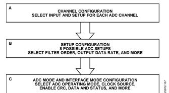
Figure 24. Suggested ADC Configuration Flow
