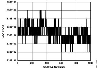
Figure 5. Noise (Output Data Rate = 1.25 SPS)
