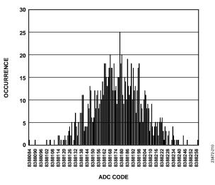
Figure 10. Histogram (Output Data Rate = 31.25 kSPS)
