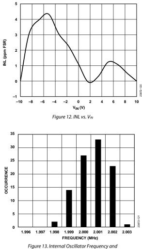
igure 13. Internal Oscillator Frequency and Accuracy Distribution Histogram
